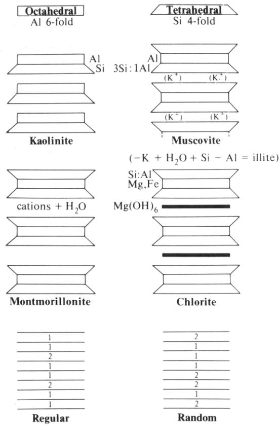
Fig. 3.10 : Mineralogy of clay material (after Pettijohn et al. 1972)
