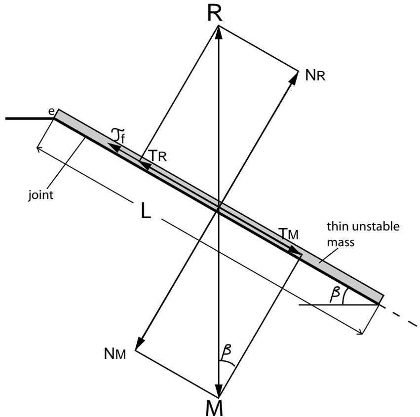
Fig.2.6 : Limit equilibrium of a slope containing a planar discontinuity (without water).
