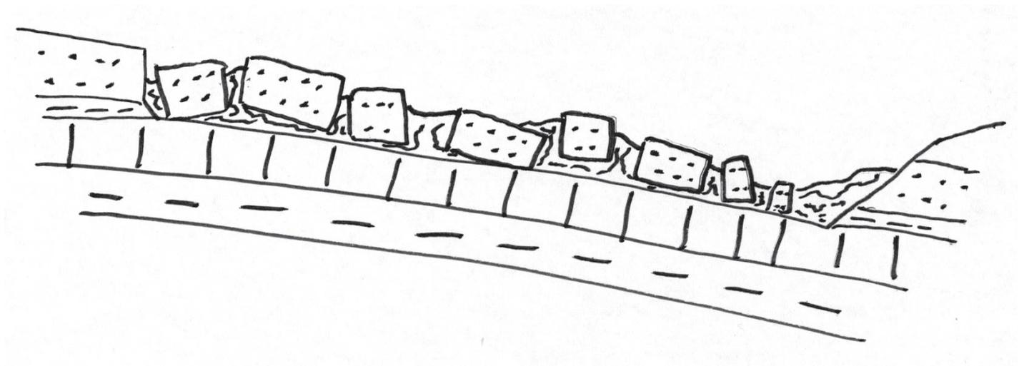
Fig. 5.4.1: Schematic profile of the spread phenomenon in a slope
