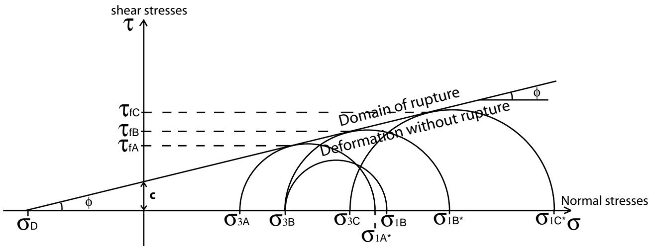
$\sigma_{1*}$  = maximum normal stress at failure
