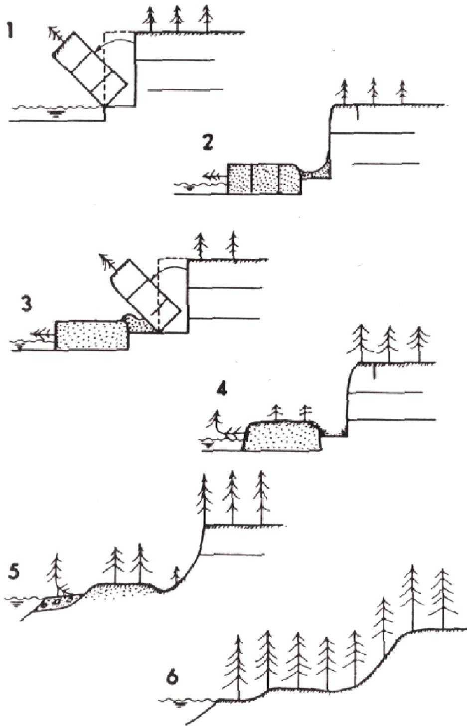
Fig. 4.3 : Degrees of activity of a landslide according to the International Glossary (Cruden and Varnes).
