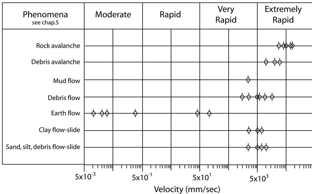
Fig.4.2 : Maximum velocities of movements for the flow type phenomena (modified from Hungr, 2001).
