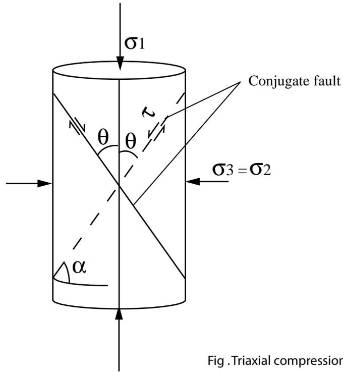
Fig .Triaxial compression test.
