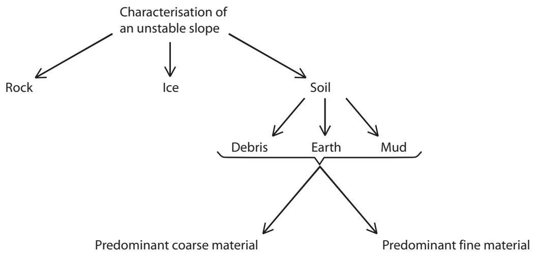
Fig. 3.4 : General categories of geological material moving in unstable slopes
