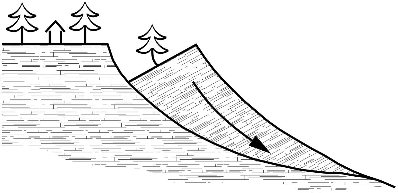
Fig. 5.3.3 : Schematic profile of a deep rotational slide.
