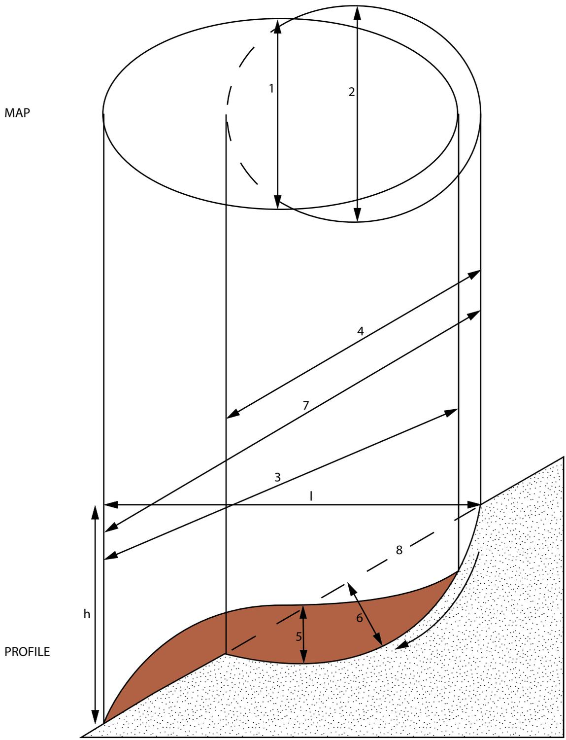
Fig. 3.3 : Geomorphological parameters of a landslide (modified from Cruden and Varnes).
