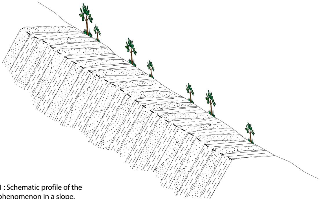
Fig. 5.2.1 : Schematic profile of the topple phenomenon in a slope.
