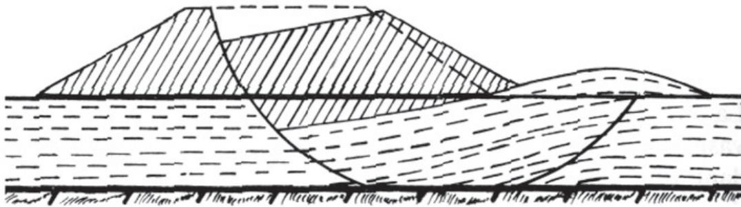
a) Standard diagram of circular rupture.
