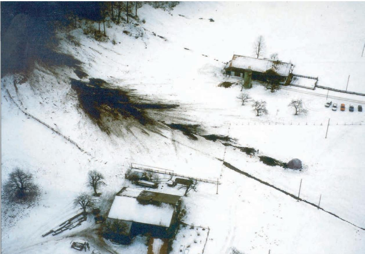
Fig. 5.1.3 : Single block-fall from a conglomerate formation in Grindelwald, Burglauenen (2.2.1994). Photo Geotest AG.
