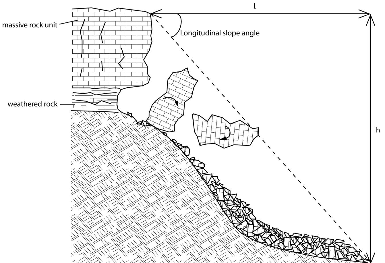
Fig.5.1.1 : Schematic profile of a rock fall from a cliff.
