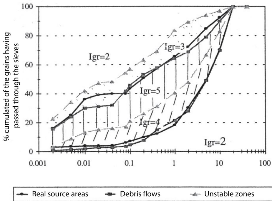
Fig. 5.5.5 : Domain of grain size distribution of unstable soils in the French Alps (Bonnet-Staub, 1999).
